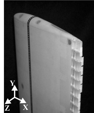
Fig. 3 Trailing edge of wing with four MiTEs actuated in down position.
